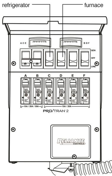
To maximize the efficiency of your generator, divide appliance circuits and others requiring higher wattage between adjacent circuit selector switches of the transfer switch so that a usage balance is achieved between the opposing legs of the generator power. For example, on a 6-circuit transfer switch, consider wiring the refrigerator to Switch C and the furnace to Switch D (*Figure 3*).
